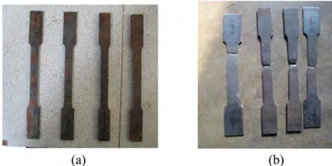
**Fig. 6.** Steel coupons used in tensile testing (a) original specimens and (b) tested specimens.
